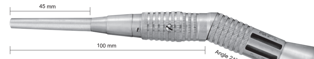
M8-211 INTRA Main Piece, Angular No key needed for tightening Tip 45 mm long Transmission: 1:2 Burrs shank: Ø 2.35 mm Burrs length: 95 mm Weight: 98 g
