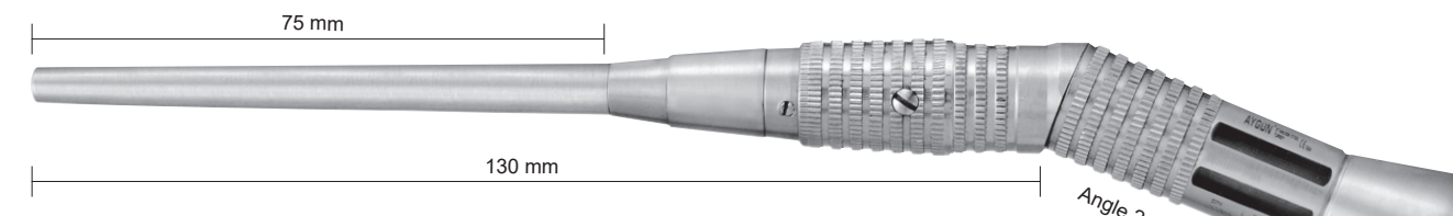
M8-212 INTRA Main Piece, Angular No key needed for tightening Tip 75 mm long Transmission: 1:2 Burrs shank: Ø 2.35 mm Burrs length: 125 mm Weight: 105 g
