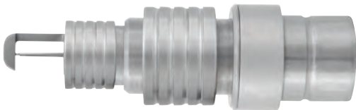
M102-255 Cranial burr attachment Dura guard, rotatable 15.000 rpm 35 x 118 mm / 320 g
