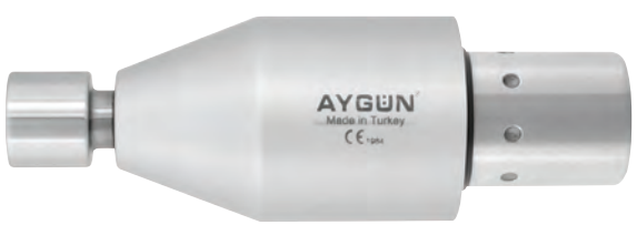
M103-970 TPLO Saw attachment (Without saw blades) 16.000 cpm / \angle 4^{\circ} 50' 42 x 120 mm / 400 g
